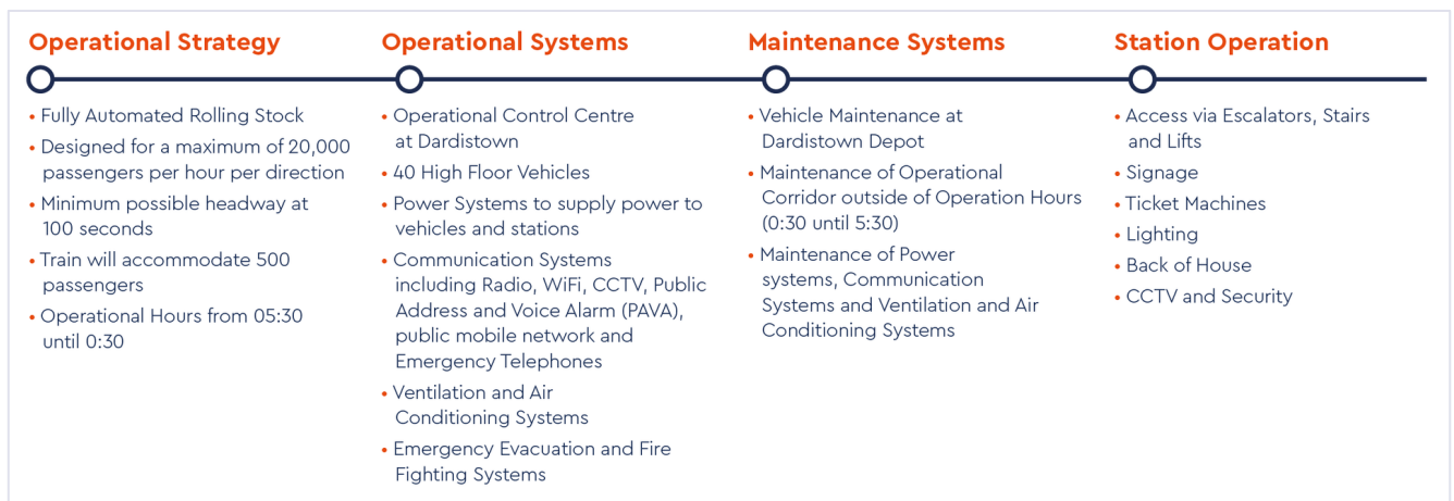
Diagram 6.2: Summary of Key Considerations during the Operational Phase of the Proposed Project
