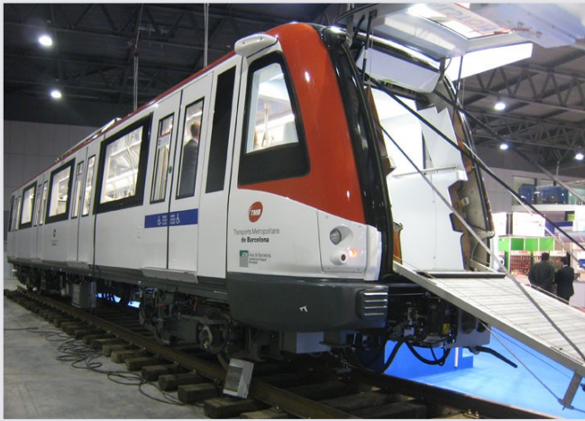
Diagram 6.8: Typical Ramp for Vehicle Evacuation
